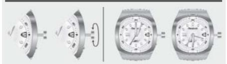
**3-Position Crown**: Pull crown to "MIDDLE" position and turn **CLOCKWISE** or **COUNTER-CLOCKWISE** until correct date appears.
